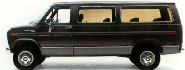
Passenger Van TRANSMISSION: 3-speed automatic ► ENGINE: V-8 ► FUEL: unleaded ► FUEL CAPACITY: 40 gallons (approx.) ► EXTRA EQUIPMENT: Power steering and brakes
